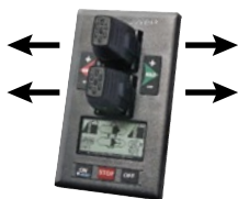
Activating both bow and stern thruster to push the boat sideways
