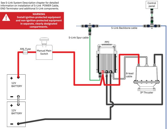
The top and bottom wiring setup is for a dual thruster system, For example bow and stern.
