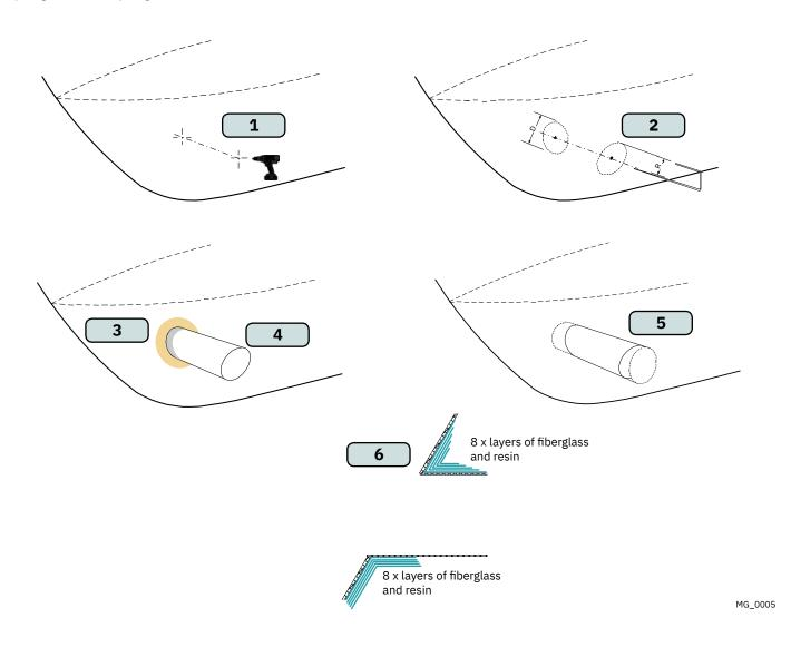
With tunnel installed and cast.
