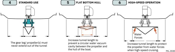
Some sail boats have a flat bottom and shallow draft in the bow section. This can make installing the thruster as far forward from the boats main pivot point difficult. (Fig. 1).
