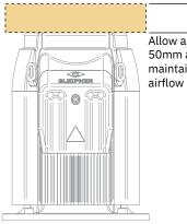
Allow a minimum of 50mm above the fan to maintain appropriate airflow to the cooling fan.
