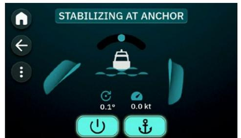
*(NB: If both Cruising and At Anchor modes are activated, the system will automatically switch between them based on vessel speed. The system will turn OFF automatically if speed drops below 3 knots and At Anchor Mode is not enabled.)*
