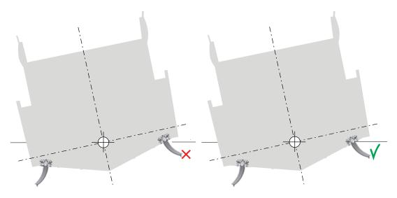
No part of the fin should be above water level during normal roll motion/under normal sea conditions.
