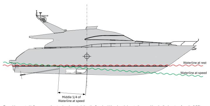
To avoid unwanted influences on the steering characteristics, the fins should be placed close to the vessel longitudinal centre of gravity (LCG) - If unknown, this is usually a little aft of 50% of the waterline length.
