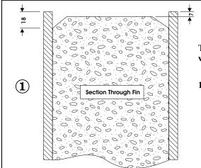
The fins are made with a pre-molded foam core with a vacuum injected Vinylester skin.
