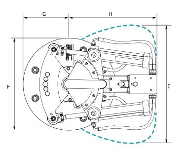
The fin actuator assembly may be installed in any convenient radial 360° position in the hull.
