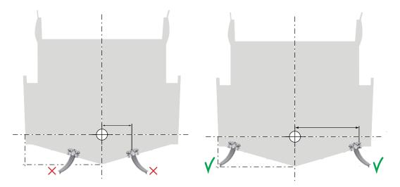
Fins should not extend outside the beam or below the keel when in neutral position.
