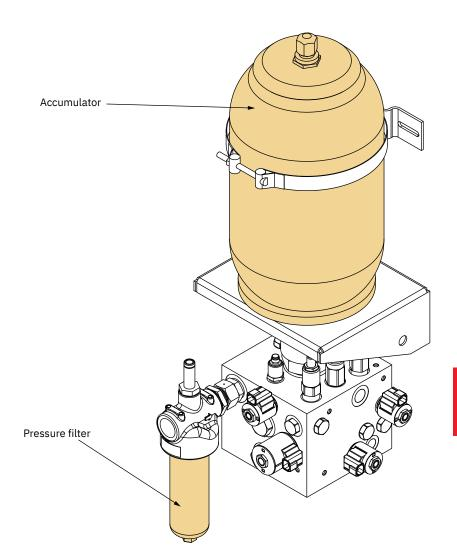
WARNING Running the system without any nitrogen/pressure on the tank will damage the stabilizer system.
