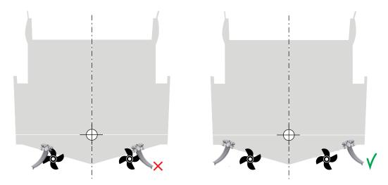
Fins should be placed as far outboard as possible, and NOT in-line with the propellers, to ensure avoiding possible disturbance of the water flow to the props which in the worst case can cause vibrations / cavitation.
